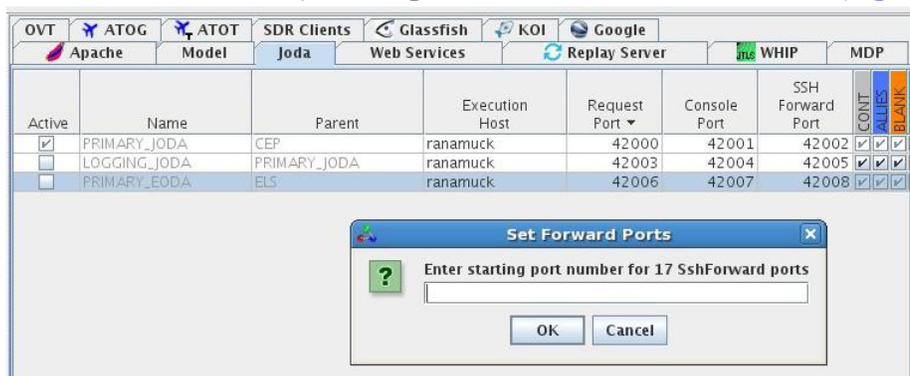
Figure 1.2 ICP SSH Forward Ports Configuration Window
